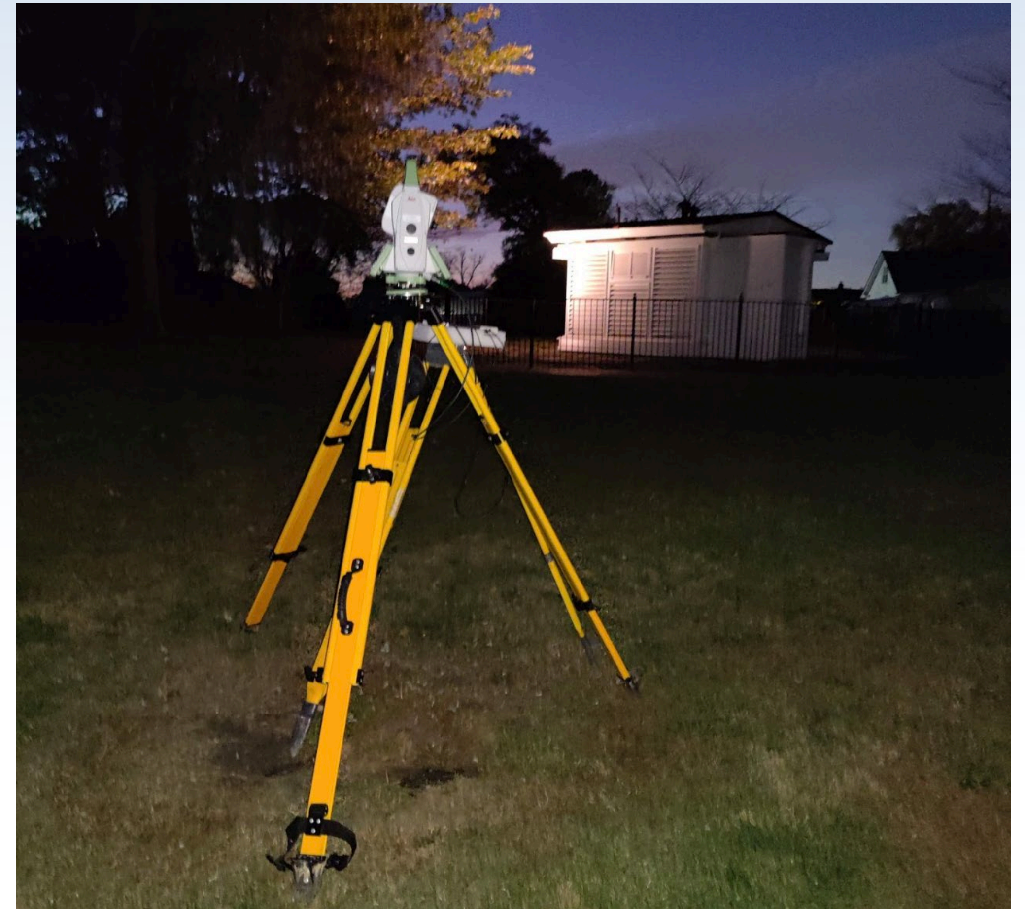
TSACS being tested at the International Latitude Observatory historical site in Gaithersburg, MD
