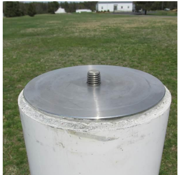
Figure 3. Forced Centering Adapter set into top of above-ground section of monument.
