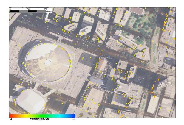
Figure S1. Close up of Superdome near downtown New Orleans from aerial photography after Hurricane Katrina (note damaged roof of Superdome), with superimposed velocity of permanent scatterers. Radar illumination from left, solar illumination from right.
