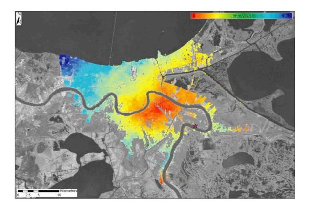
Figure S2. Standard deviation of individual permanent scatterers. Star marks location of GPS calibration point ENG1.
