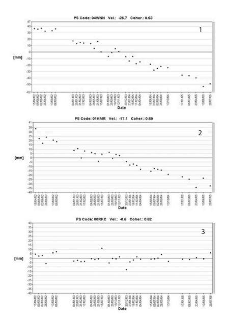
Figure S3. Time series of several individual permanent scatterers. Each point represents data for an individual pixel from an individual SAR image (total 33). Points 1 and 2 are on the levee bounding the MRGO canal, point 3 is within 1 km of the GPS calibration point.
