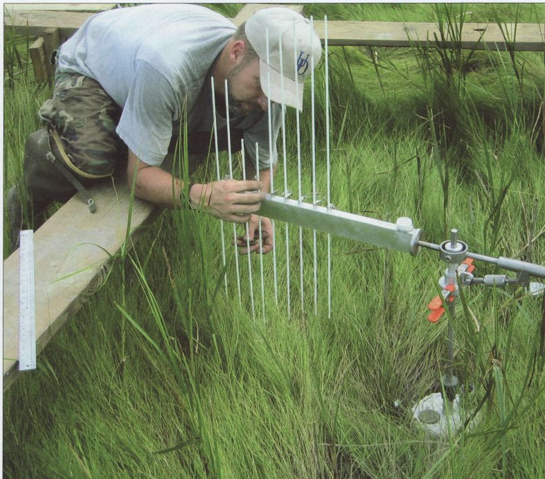
Figure 1: The deep rod SET as deployed on top of a SET benchmark in a coastal salt marsh. (Photo courtesy of D.R. Cahoon, US Geological Survey).
