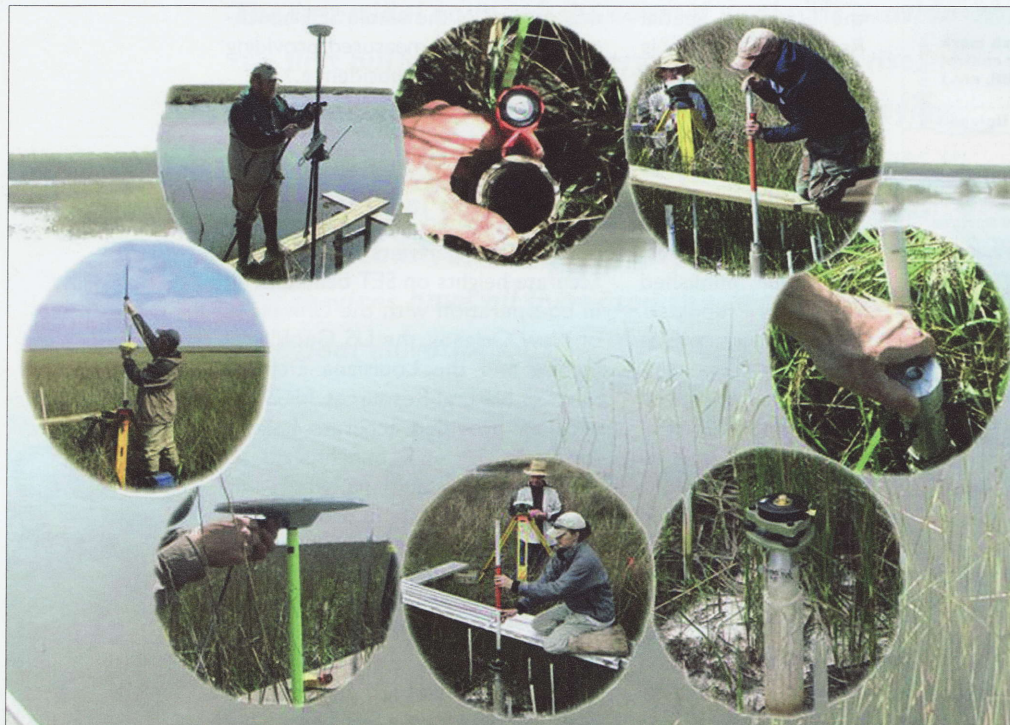
Figure 4: Protocols for tying SET benchmarks to the National Spatial Reference System. Clockwise from top: locating top of SET benchmark pipe; levelling to top of pipe; installing tribrach adapter; tribrach installed; levelling to top of tribrach; installing GPS antenna; installing RTK-GPS base station; obtaining elevation using RTK. Artwork courtesy Bob Leonard, NOAA NGS.
