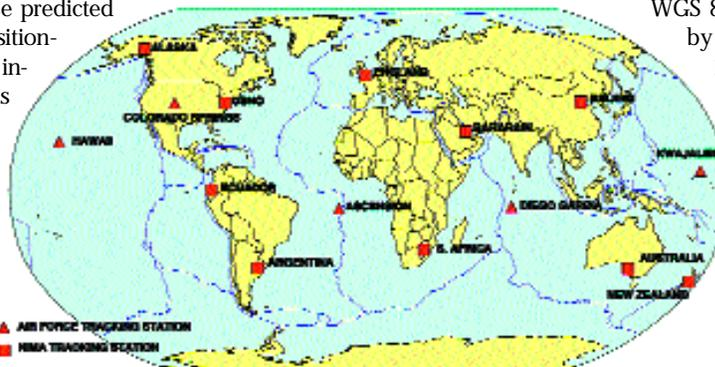
Figure 3. Combined DoD tracking network that defines WGS 84.
