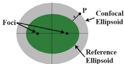
Figure 8: Illustration of the concept of two gravitationally-equivalent confocal ellipsoids.
