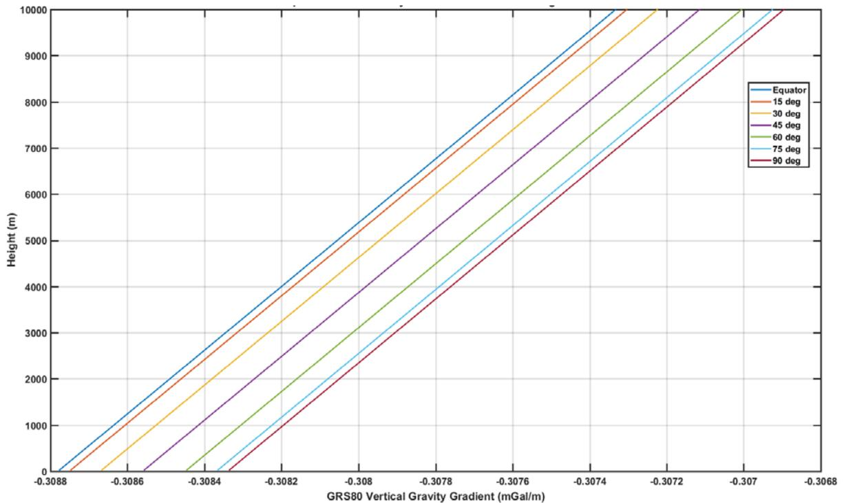
Figure 7: GRS80 ellipsoid vertical gravity gradient variation with respect to latitude and height above the ellipsoid surface.
