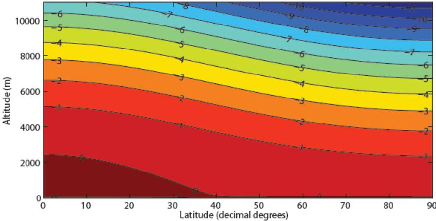
Figure 8: Difference (mGal) between the 1st order (linear) free-air correction and a comparable correction derived from the confocal ellipsoid computation of normal gravity at any height with WGS84.
