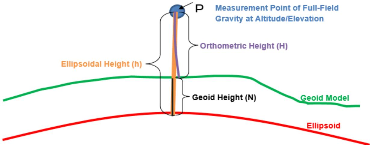
Figure 5: Sketch (not to scale) of the difference between orthometric height (height above the geoid), ellipsoidal height (height above the ellipsoid), and geoid height (height of geoid above ellipsoid).
