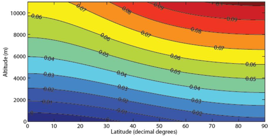
Figure 6: Difference (mGal) between the 2nd order free-air correction and a comparable correction derived from the confocal ellipsoid computation of normal gravity at any height with WGS84.
