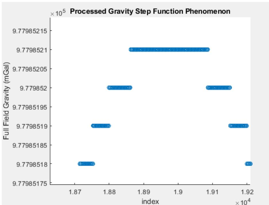
Figure 4: Discontinuous Step Function Phenomenon with 20 Hz Gravity Data.
