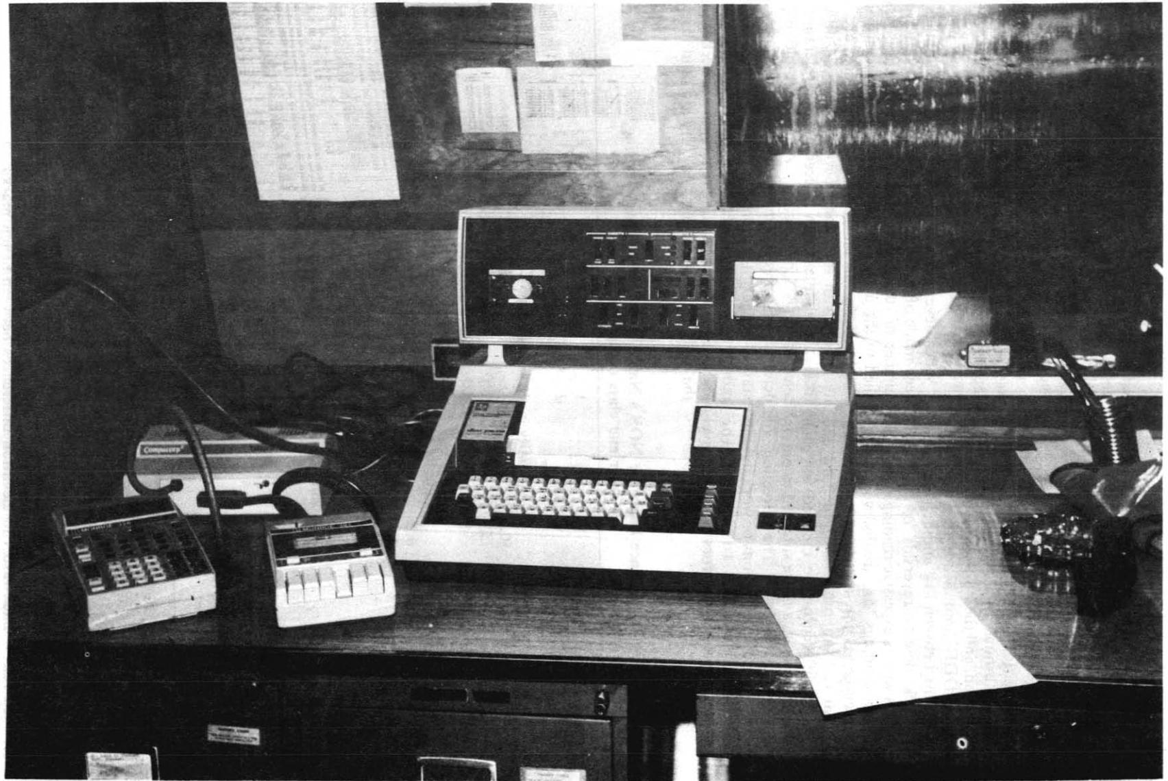
Figure 7.—Monroe 326 calculator and 392 recorder, Compucorp 396 interface unit, and Texas Instruments programmable terminal.
