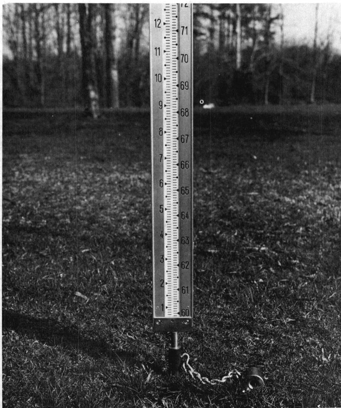
Figure 6.—Kern 0.5-cm double-scaled rod on turning pin.
