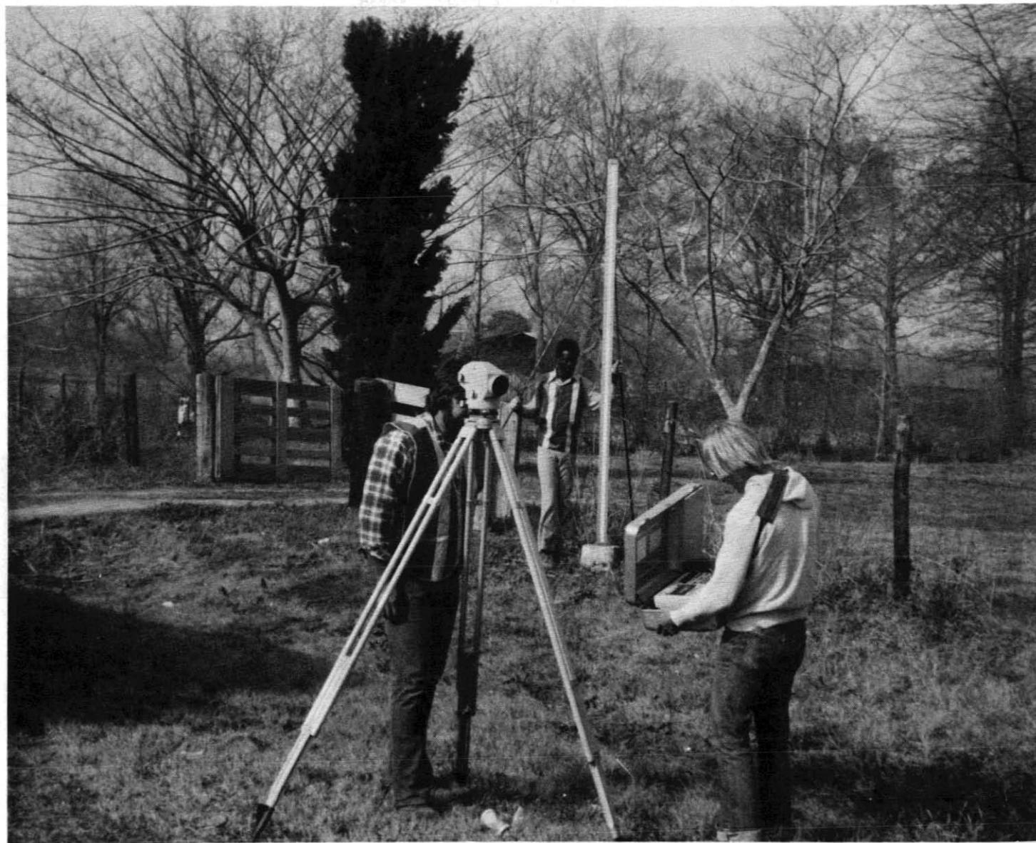
Figure 4.—Magyar Optikai Muevek (MOM) NI A 31 compensator level in operation .
