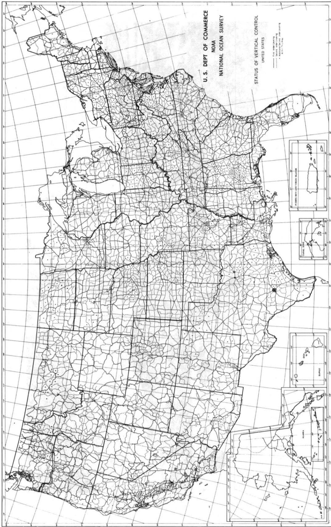
Figure 1.—The United States geodetic vertical control net.
