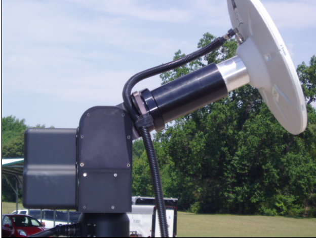
Figure 2: Two-axis robot used to move the antenna under test, shown here with a Trimble Zephyr Geodetic II antenna and 20-cm extension to separate antenna from the robot body.
