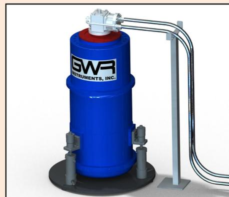
Rendering of Field SG showing base plate with leveler, Dewar and coldhead
