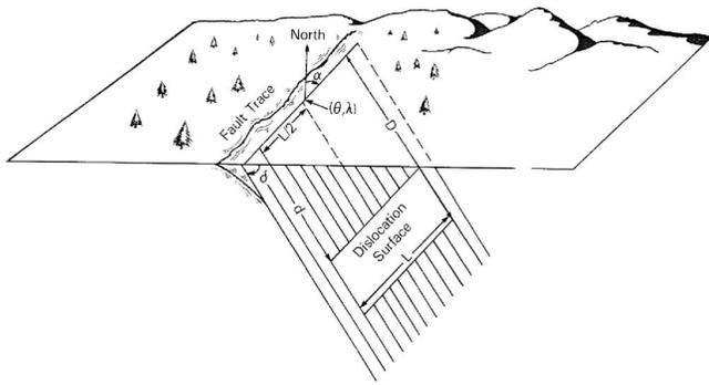
**Fig. 2.** Schematic diagram of a dislocation. The rectangle represents the dislocation surface or slipping patch on a fault. The deformation measured on the surface depends on the strike ( $\alpha$ ) and dip ( $\delta$ ) of the fault plane, the length of the dislocation ( $L$ ), the depth to the top ( $d$ ) and bottom ( $D$ ) surface of the dislocation measured along the fault plane and the latitude and longitude ( $\theta$  and  $\lambda$ ) of the fault center.
