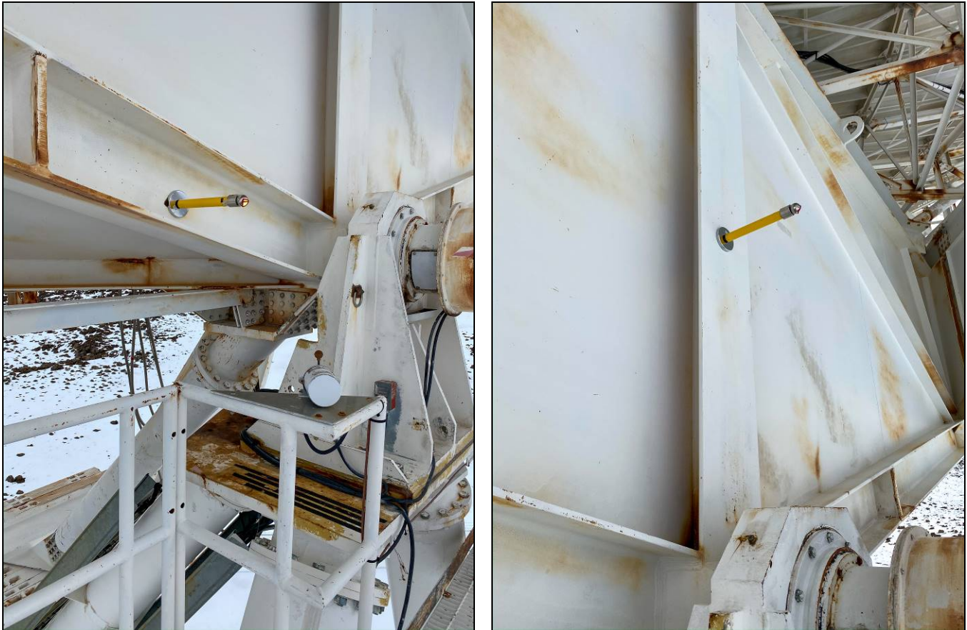
Target/reflector affixed to VLBI antenna for elevation and azimuth rotation sequences
