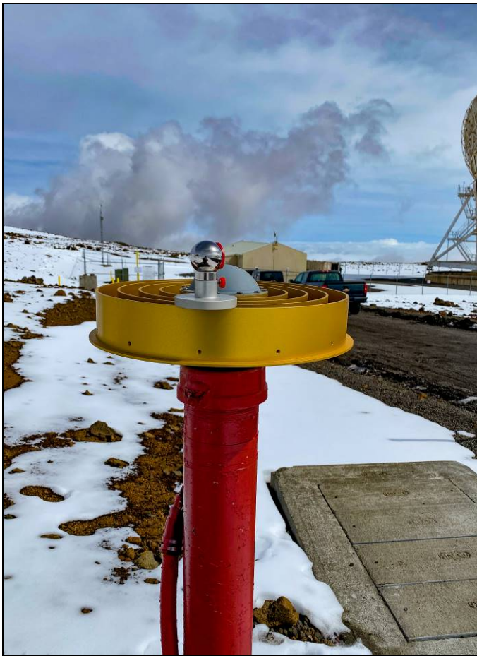
Observations of the choke ring were used to determine the GNSS reference point through circle-fitting
