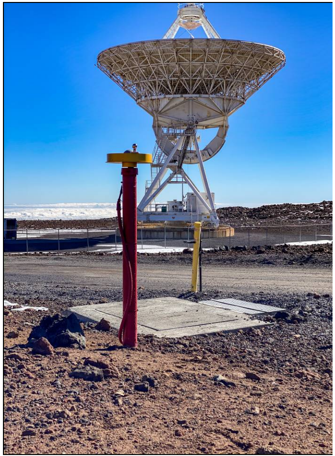
Observations of the choke ring were used to determine the GNSS reference point through circle-fitting
