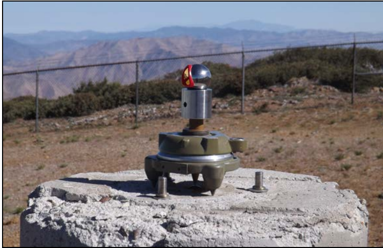
Figure 3 – Kern trivet on DORIS mark.
