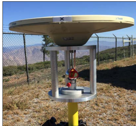
Figure 2 – MTA with attached optical reflector and GPS antenna.
