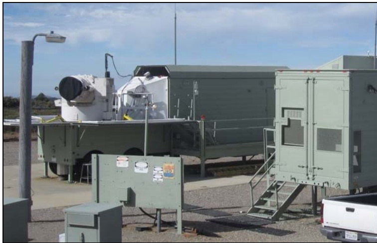
Figure 11 – SLR instrument MONL
