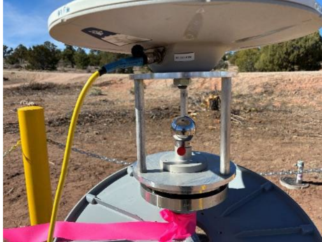
SCIGN Mount at PTV2 with MTA and GNSS Antenna
