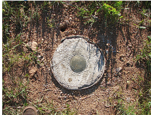
Figure 4 – Ground network mark TMGO RM 1
