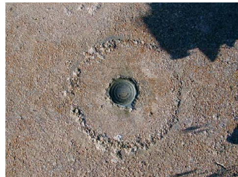
Figure 2 – Ground network mark BOULDER CG
