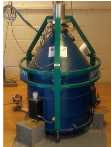
Figure 7 – NGS SC gravimeter set up over IRM. The circle offset bar with prism can be seen to the left of the SG.
