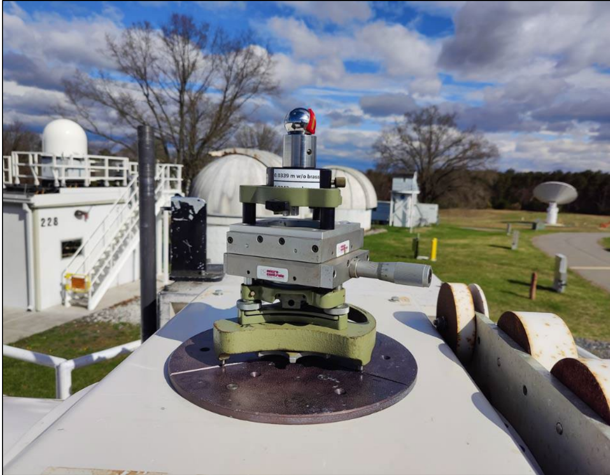
2-dimensional translation stage mounted on MOBLAS-7
