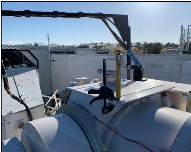
MOBLAS-7 with mounted reflector. Targets were positioned as they scribed circles about the azimuth and elevation axes.
