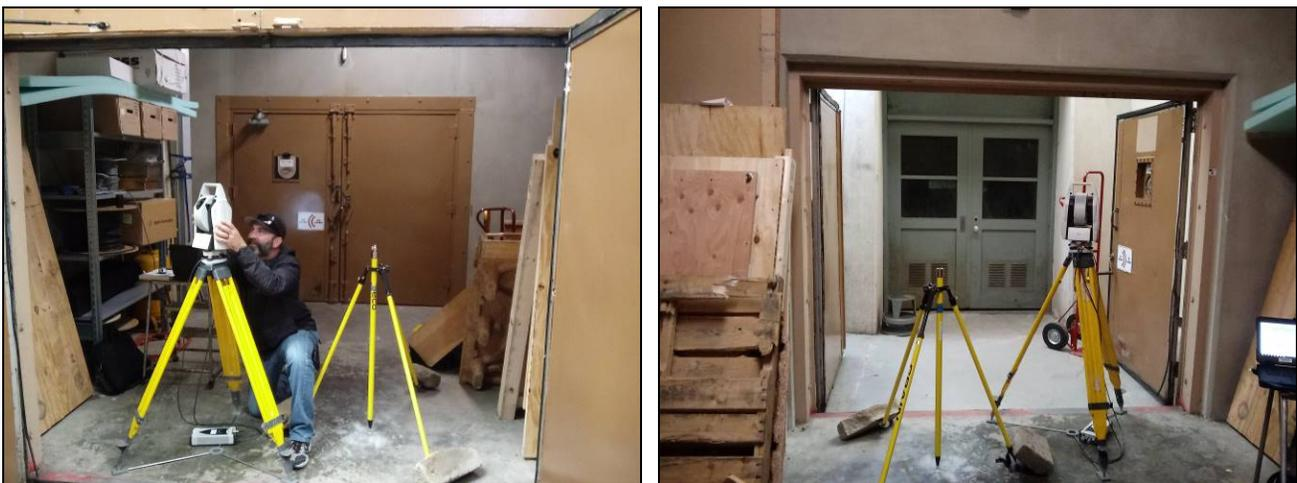
Laser tracker setup and mark NGS A, inside the airlock to extend the survey network into the VLBI telescope's radome structure
