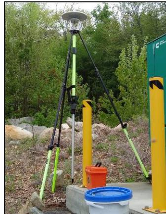
Fixed-height range poles for reflectors and GNSS antennas
