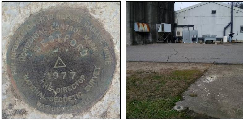
**WESTFORD RM1** is a National Geodetic Survey reference mark disk, stamped WESTFORD NO 1 1977, cemented in a drill hole in a 2 foot square concrete slab that projects 4 inches above the ground surface. The datum point is a cross in the center of the disk.
