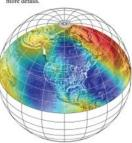
The new datums will extend across CONUS and U.S. tretrieories. The geometric datum replacing NAD 88 will be consistent with geocentric glabal reference frames defining latitude and longitude. The geopotential datum replacing NAVD 88 will be based on a gravitority good model, enhanced by data from NGS Gravity for the Redefinition of the American Vertical Datum (GRA-VD) Project.
