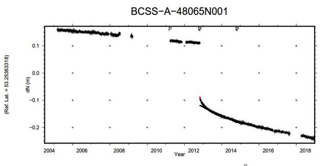
Time series showing crustal motion following the Haida Gwai earthquake of 2012. Velocities and uncertainties estimated using in-house SINEX combination software.
