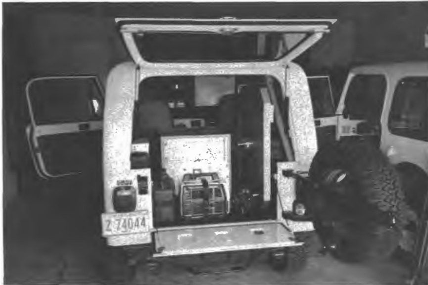
Figure 4. -- Macrometer receiver installed in a jeep vehicle. Equipment accessories shown include the antenna, tripod, and generator.
