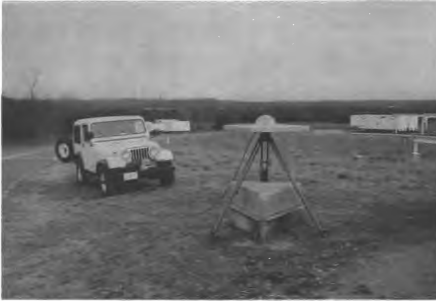
Figure 2. -- Occupation of station NORTH GEOS GORF located at Goddard Optical Research Facility, NASA, Greenbelt, Md., with the Macrometer model V-1000.
