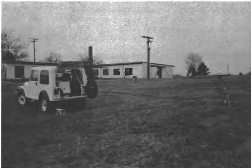
Figure 1. -- Occupation of station OPTRACK 1966 with Macrometer model V-1000 Interferometric Surveyor.
