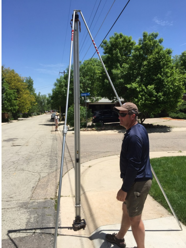
Figure 4. Leveling example. One rod is clearly visible in the foreground, the leveling unit is visible further down the street, and the far rod is just visible behind that.
