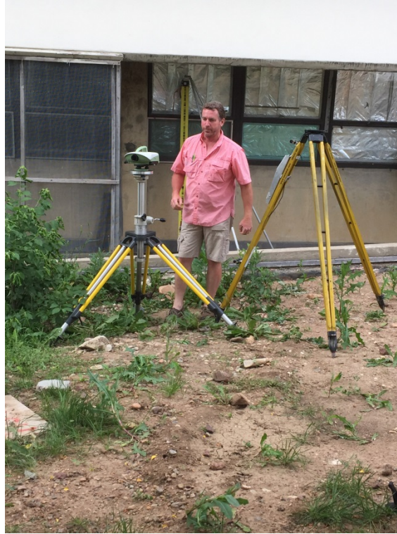
Figure 6. Leveling operations near Q407 (north side of Building 1). Q407 is visible on the wall just above the leveling unit.
