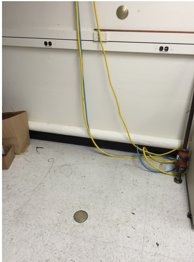
Figure 3. Examples of a floor and wall mark in the F1 clock laboratory (ATOMIC1 and ATOMIC1V).
