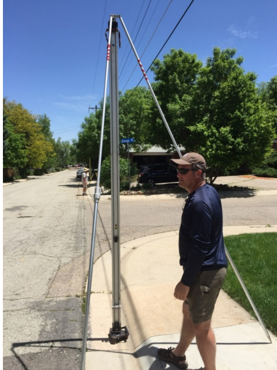
Figure 6. Leveling example. One rod is clearly visible in the foreground, the leveling unit is visible further down the street, and the far rod is just visible behind that.
