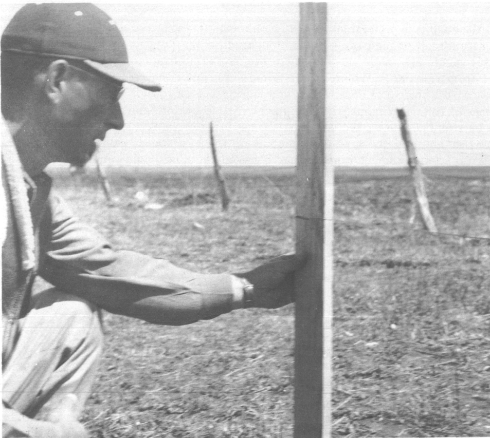
FIGURE 113.—Middle tape support on nail.
