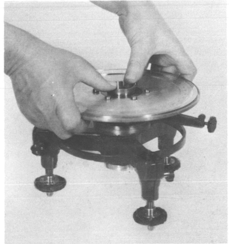
FIGURE 14.—Disassembly of circle bearing, step 2. Place thumbs on top of socket and press up on under side of circle, keeping palms of hands off the graduated surface.
