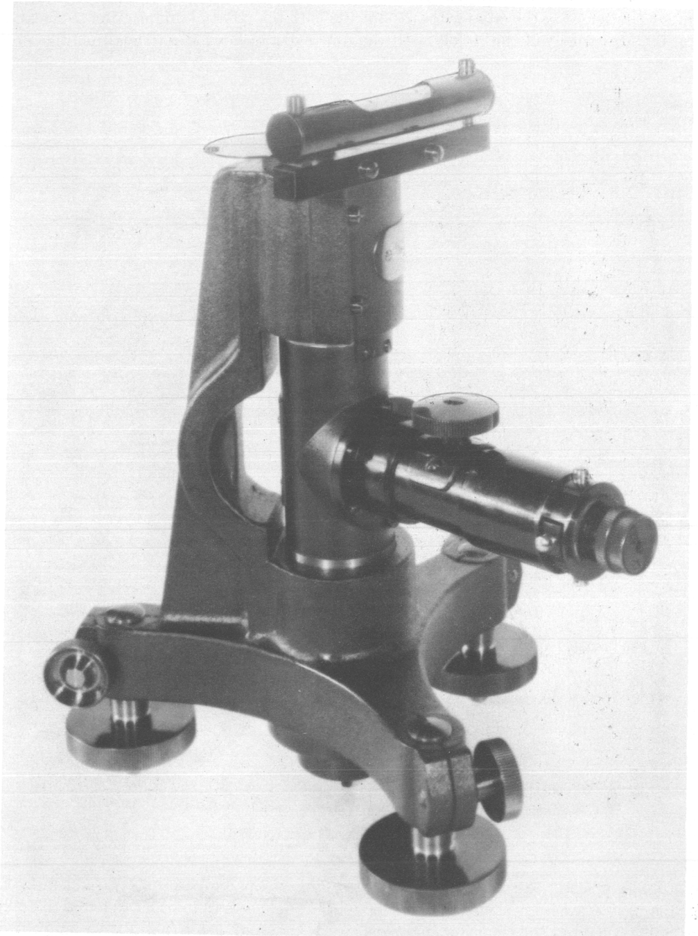
FIGURE 24.—Vertical collimator. This instrument is centered and leveled on the ground over the station mark. The telescope projects a vertical line of sight by which the light plate and theodolite on the tower are centered.
