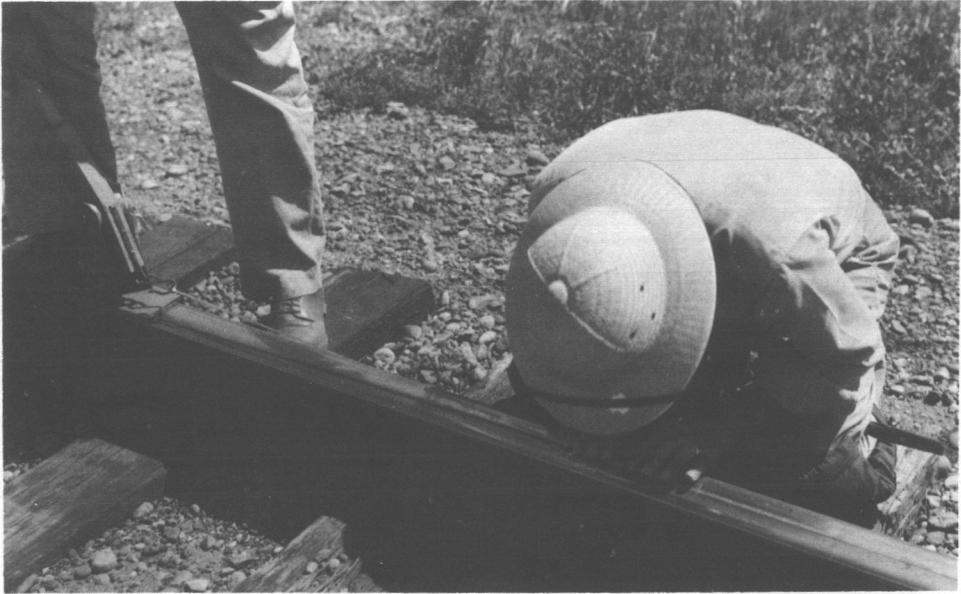
FIGURE 119.—Rear contact, base measurement on rail.
