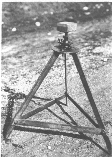
FIGURE 111.—Portable iron tripod for tape support, single joint. The wooden marking table, which carries a strip of copper on which the mark for the tape end is made, can be placed on correct slope by the ball-and-socket base and then clamped in position.
