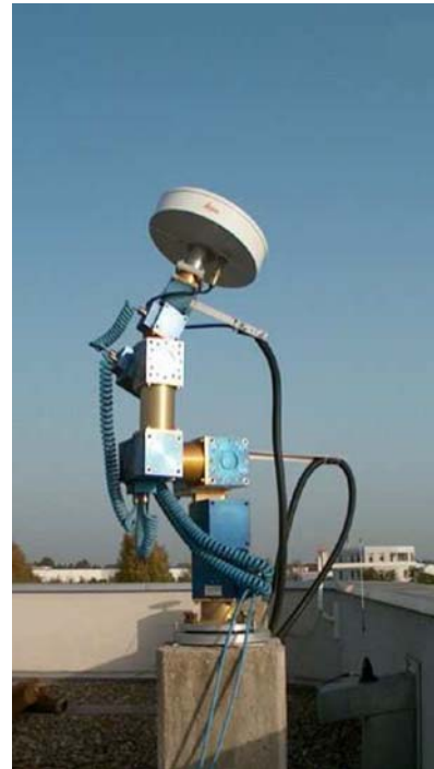
Fig. 2 Robot calibration system (Ife/GEO++) (from Wübbena et al. 2003)
