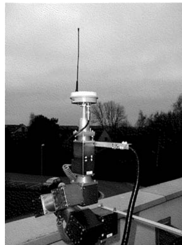
Fig. 4 DSNDGU_002_UHF* during absolute calibration using the robot
