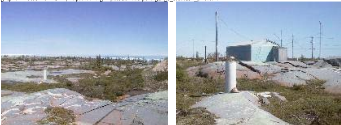
Figure 3: Site photographs of CHUR, Churchill, Manitoba, with the GPS antenna located on the ~1.5m tall pillar in both photos. Left: view to the north and Hudson Bay. Right: view to the south with metal building.
