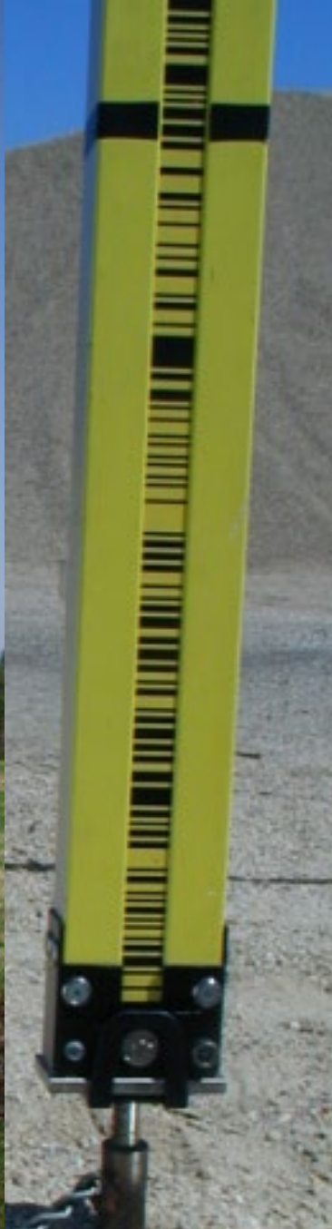
Single-Piece, Bar-Coded Invar, Calibrated Rod with Brace Poles
