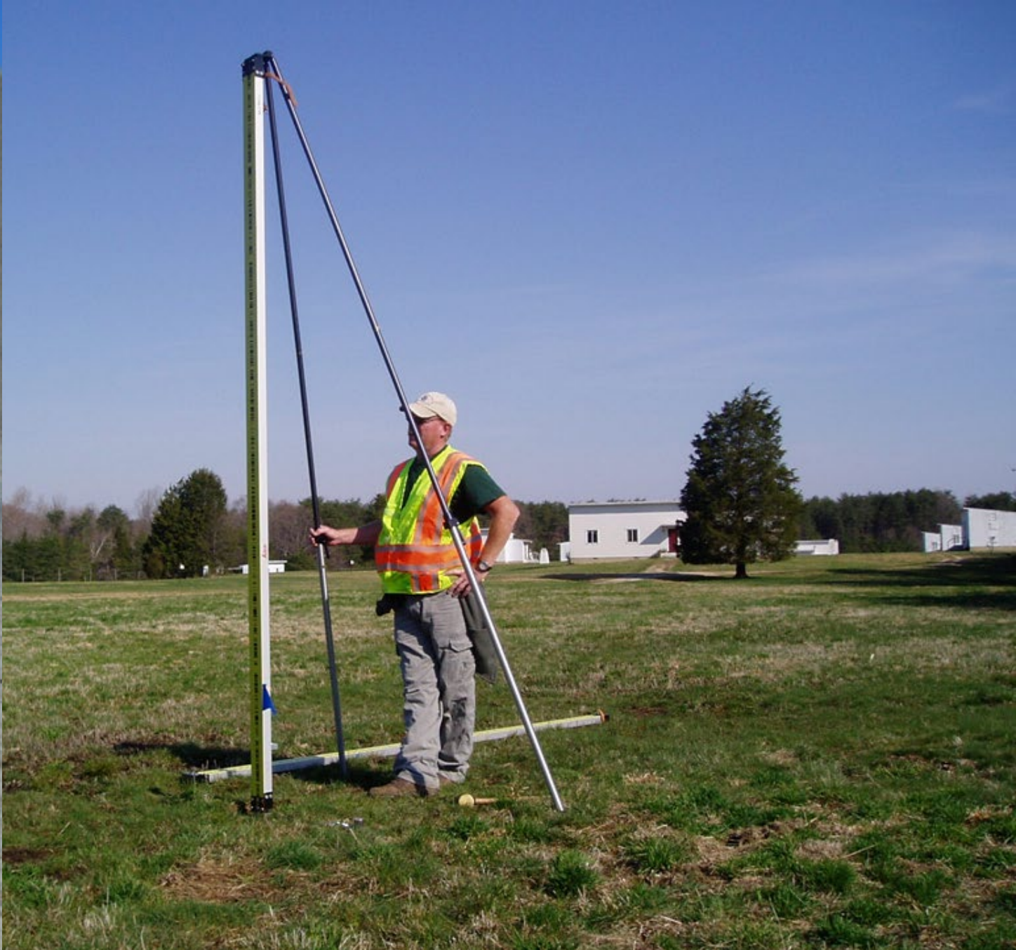
Single-Piece, Bar-Coded Invar, Calibrated Rod with Brace Poles
