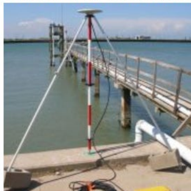
A reference mark for a water level measuring gauge
