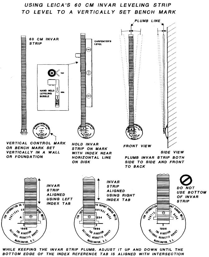
BOTTOM EDGE OF THE INDEX REFERENCE TAB IS ALIGNED WITH INTERSECTION OF THE HORIZONTAL AND VERTICAL LINES ON THE VERTICAL CONTROL MARK. USE TWO PEOPLE TO PERFORM THIS PROCEDURE. ONE CAN HOLD AND PLUMB THE INVAR STRIP, WITH THE OTHER ADJUSTS THE INDEX TO THE BENCH MARK. DO NOT USE THE BOTTOM OF THE INVAR STRIP AS THE REFERENCE POINT. USE ONLY THE BOTTOM EDGE OF EITHER OF THE TABS ON THE INVAR STRIP INDEX. (DRAWN BY ORLAND W. MURRAY, NGS)
