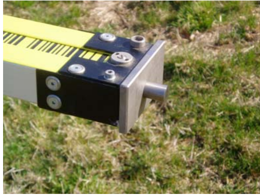
Figure 11: 2 centimeter Magnetic Spacer (“Plug”) on the base of the 3 meter rod
