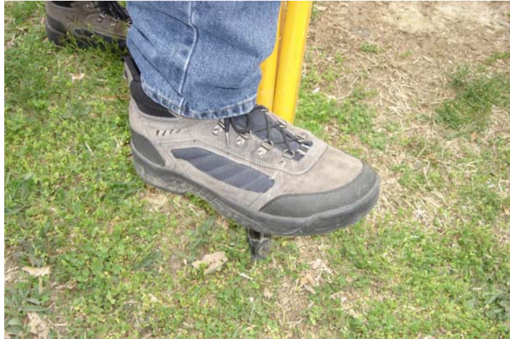
Figure 5: Pushing the feet of the tripod into the ground
