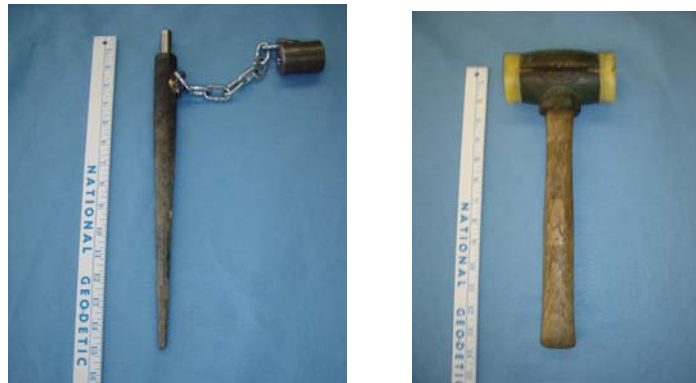
Figure 9: Steel Turning Pin and Driving Cap with Mallet with Plastic Heads For Specifications see Appendix C
