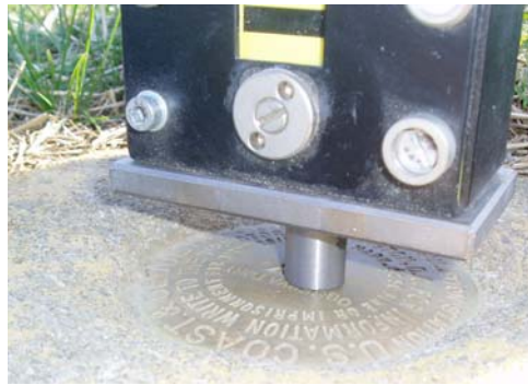
Figure 12: 2 centimeter Spacer used on a recessed bench mark
