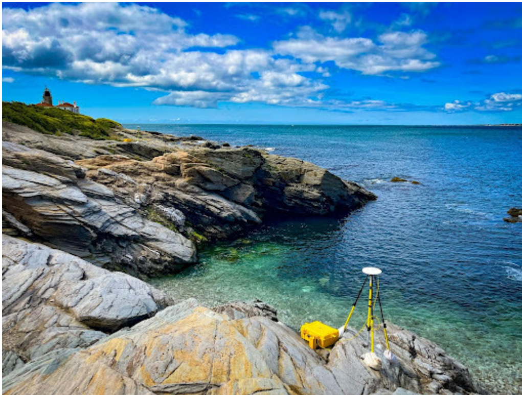
Photo: Collection of GNSS data to support VDATUM in Beavertail State Park, Rhode Island
