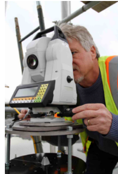
Surveyor at the top of the Washington Monument in Washington, D.C., for a 2014 survey to determine the precise position of the monument's peak.
