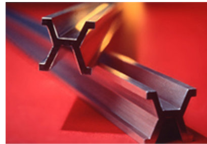
Platinum-iridium meter bars used as the standard of length in the U.S. from 1893 to 1960 (credit: NIST)
