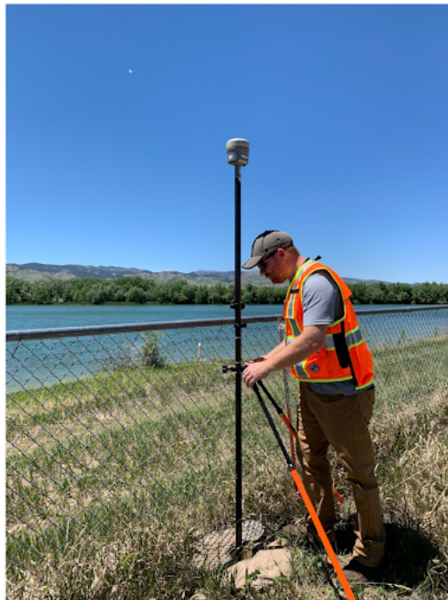
Ben Gavin, NGS, observes kinematic GPS. These observations can be completed in minutes, versus hours for traditional static GPS.
